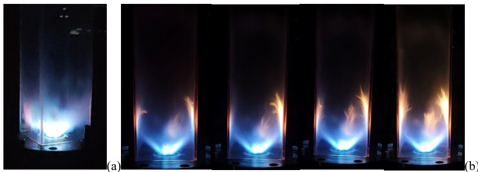
Figure 8. The swirl-stabilized atmospheric TARS burner being operated with (a) Jet A1, and (b) FAME at Re=27,000 , at \phi=0.40, 0.45, 0.50, \text{ and } 0.55 .
