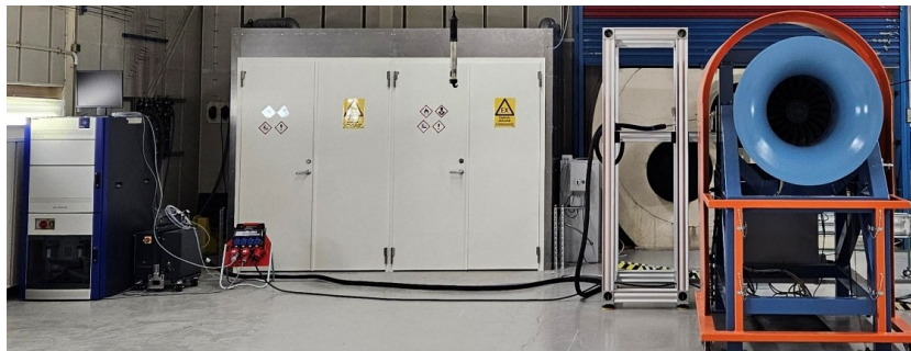
Figure 11. To the right, the turbofan engine is seen with its blue bellmouth. To the far left is the AVL AMA i60 emission analyzer, and in the middle is the enclosure for fuel storage and preparation.
