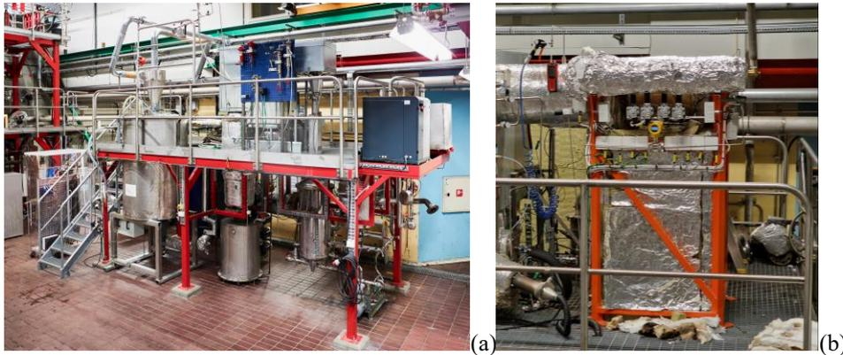
**Figure 13.** (a) Pyrolysis pilot plant before installation of hot gas filter, and (b) newly installed hot gas filter.
