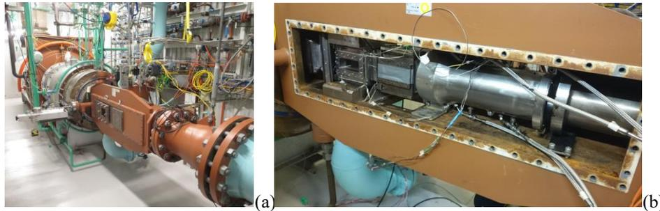
**Figure 3.** (a) DESS high-pressure combustion facility. The combustion chamber (b) with optical access is seen in the center. The parts being refurbished are mainly located downstairs in the compressor room.
