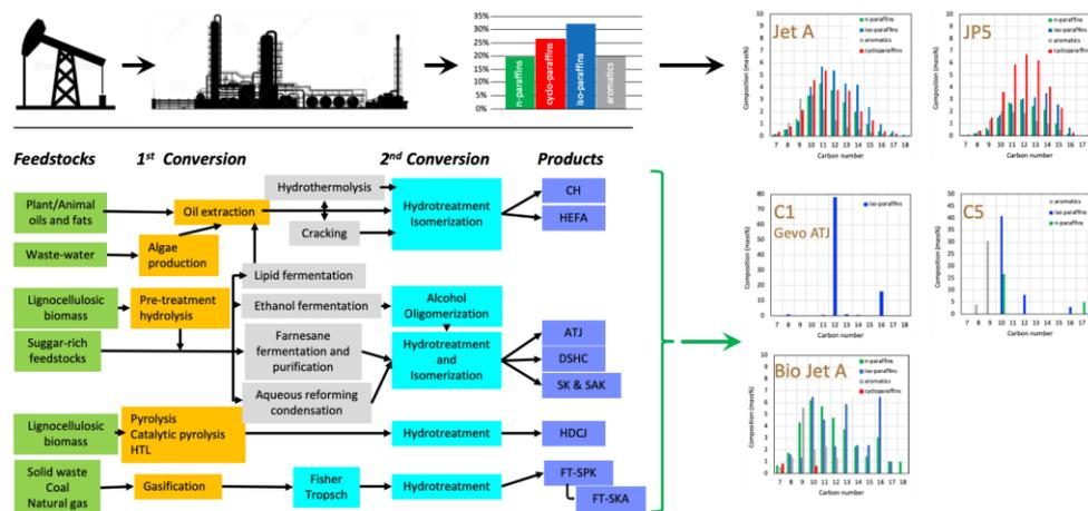
**Figure 1.** Schematic of fossil and alternative jet fuel production pathways and selected compositions of both fossil jet fuels (Jet A and JP5) as well as three alternative jet fuels.
