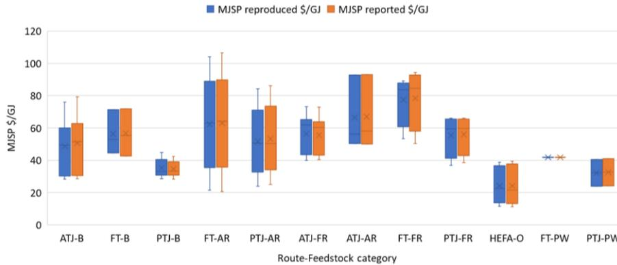
**Figure 17.** Reported and reproduced SAF production cost, Farooq *et al.* (2023, manuscript under preparation). AR – agricultural residues, FR – forest residues, O – oil feedstock, PW – process waste, B - other lignocellulosic biomass, ATJ - alcohols-to-jet, PTJ - pyrolysis-to-jet, FT -- gasification + Fischer-Tropsch, HEFA - hydroprocessed esters & fatty acids.
