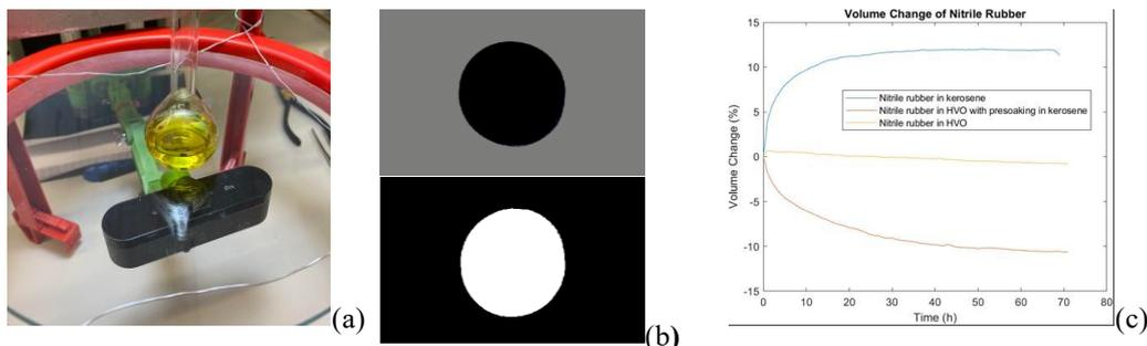
**Figure 16.** (a) Set up of optical dilatometer. (b) Image processing of o-ring cross sections. (c) Example nitrile rubber elastomer fuel swelling graph.
