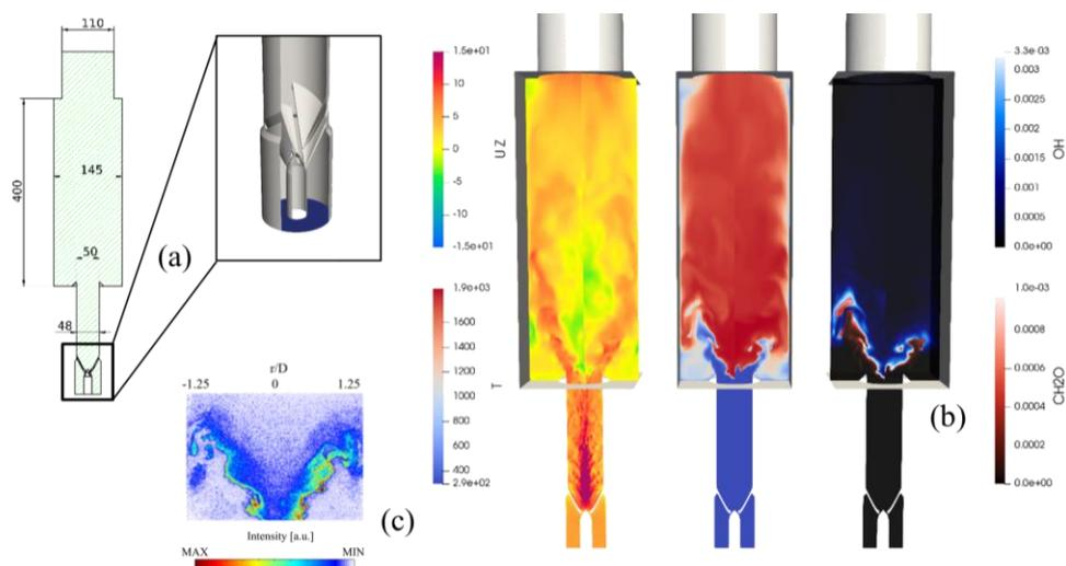
**Figure 15.** (a) Main geometrical elements of the CECOST burner, and a detail of the axial swirler. (b) From left to right: axial velocity, temperature and OH/CH<sub>2</sub>O distributions (blue and red) for PaSR and EDC in the two halves of the combustion chamber (left and right, respectively). (c) Instantaneous experimental OH\* PLIF signal.
