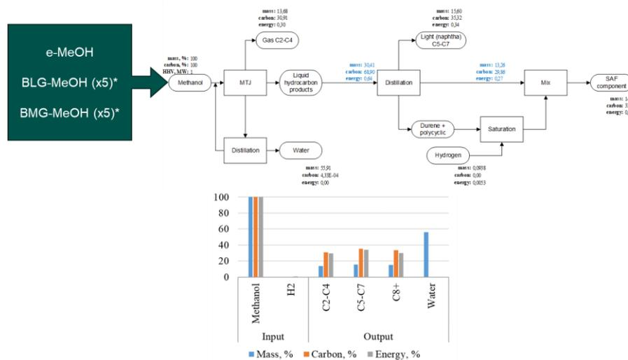
**Figure 18.** Schematics for SAF production via methanol-to-jet track used for the techno-economic evaluation. e-MeOH – captured CO<sub>2</sub> based methanol (via a reverse water-gas-shift process), BLG-MeOH – Black liquor gasification-based methanol, BMG-MeOH – Biomass gasification-based methanol.
