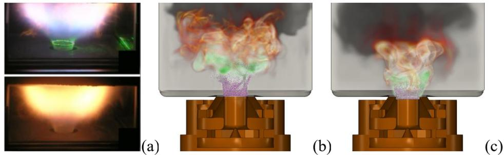
**Figure 11.** (a) Photographs of the Timecop flame at idle (top) and cruise (bottom) conditions together with numerical predictions of the spray (pink) and vaporized fuel (green), heat release (orange) and CO<sub>2</sub> distribution (gray) at (b) idle and (c) cruise conditions.
