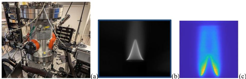
**Figure 4.** (a) Small high pressure laminar flame speed test facility, together with two different examples, (b) and (c), of laminar flame images.
