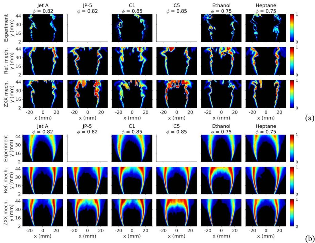
**Figure 10.** Instantaneous (a) and time-averaged (b) CH<sub>2</sub>O distributions from the experiments, [6], (top row), small, detailed reaction mechanisms (middle row) and the pathway centric reaction mechanisms (bottom row).
