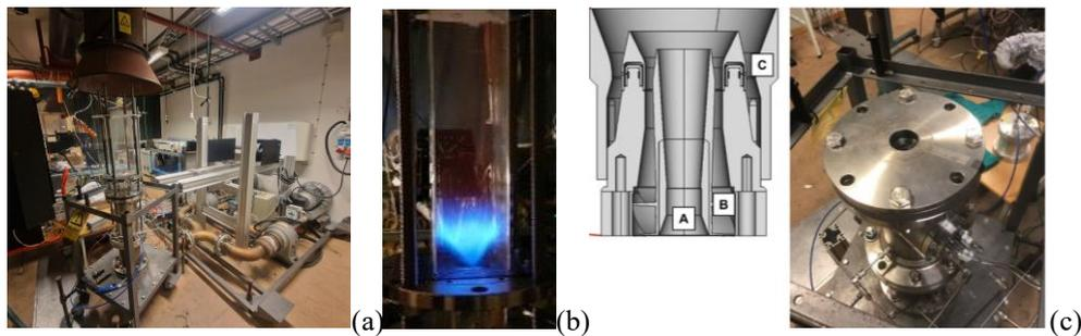
**Figure 5.** (a) the atmospheric combustion test facility, (b) the CECOST burner in operation with gaseous fuel, and (c) a schematic and the hardware of the TARS burner.
