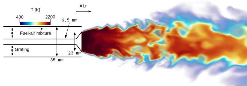
**Figure 9.** Schematic of the geometry, along with a volume rendering of temperature obtained for Jet A. Note that the pipe is mounted vertically in reality.
