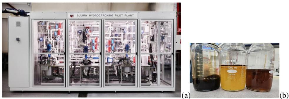
**Figure 14.** (a) Slurry hydrocracking pilot plant. (b) Samples of heavy oil product (left), aqueous product (middle) and light oil product (right) from stabilization of the produced pyrolysis oil.
