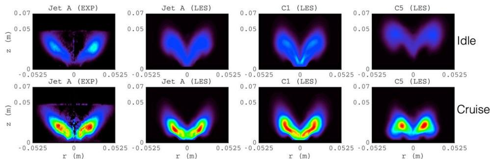
**Figure 12.** Time-averaged OH chemiluminescence images from the experiments (left panels) of Jet A compared with corresponding numerical images from Jet A, C1, and C5.
